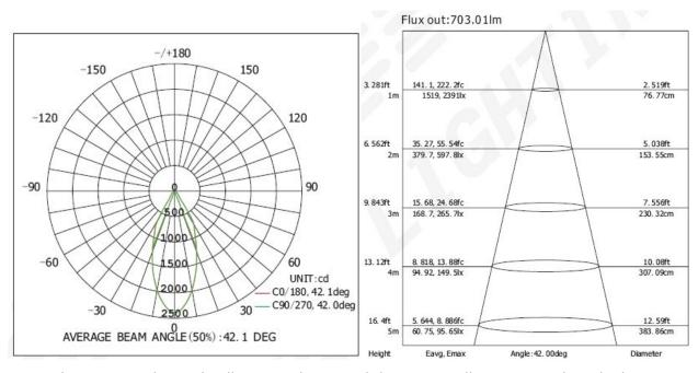
Note: The Curves indicate the illuminated area and the average illumination when the luminaire is at different distance.
