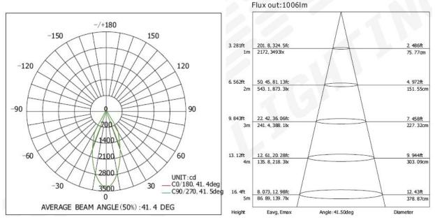
Note: The Curves indicate the illuminated area and the average illumination when the luminaire is at different distance.
